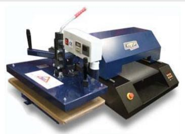
The PreJet is the first digital printer in the world specifically developed for the application of Pre Treatment Solution for textile decoration. Applying Pre Treatment Solution by use of inkjet technology offers many advantages to the traditional manual application method.
