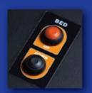
**BUTTONS** - Micro-step platen height adjustment.
